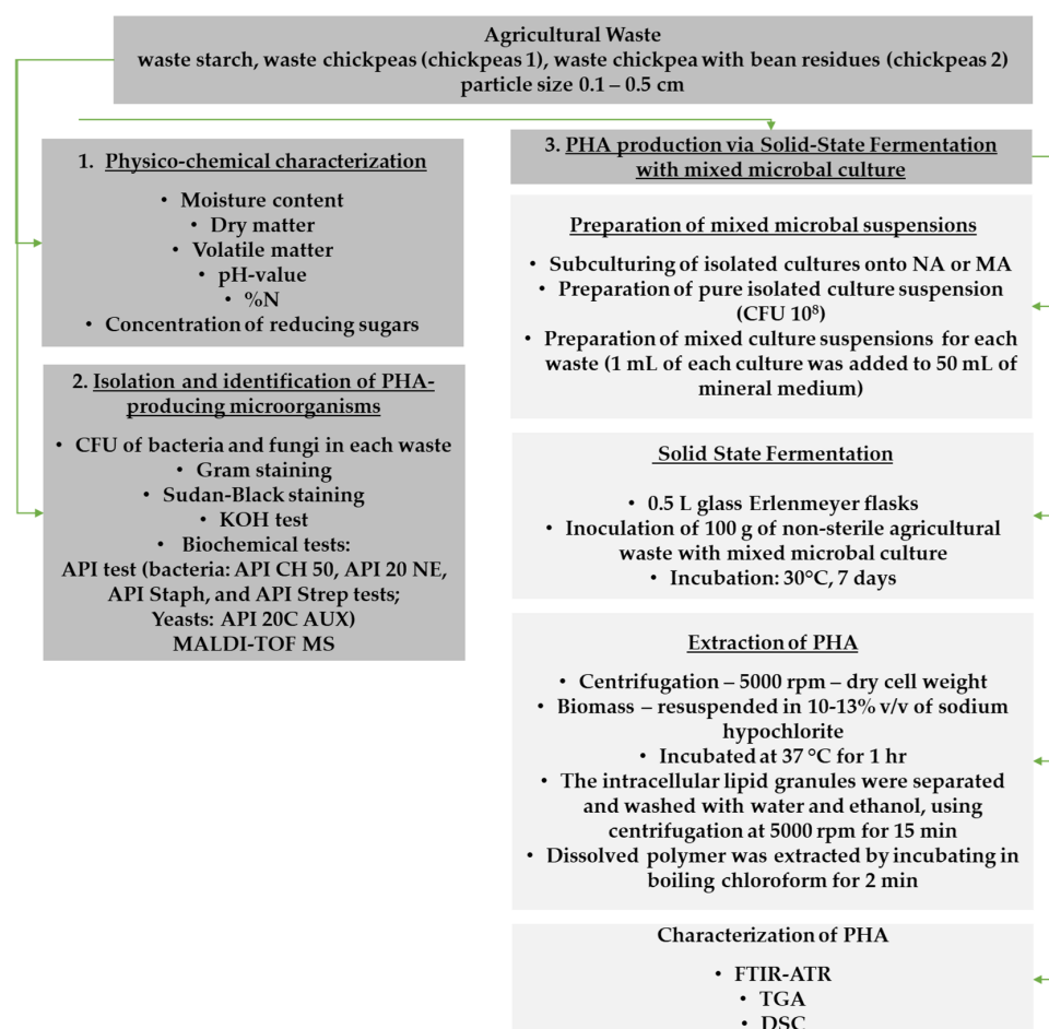
Figure 1. Experimental workflow for PHA production.
